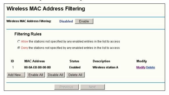
Figure 4-14 Wireless MAC address Filtering
